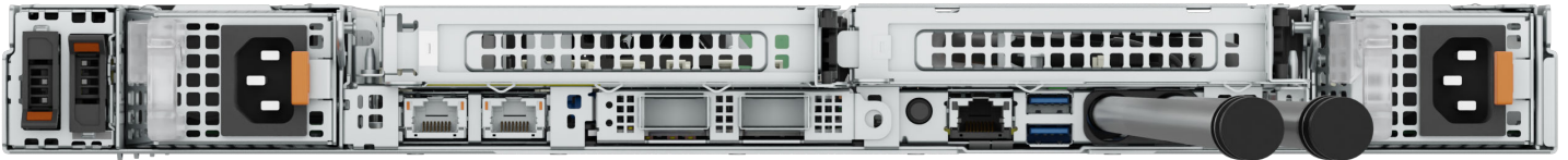
Figure 8. Rear view of the system with Direct Liquid Cooling module
